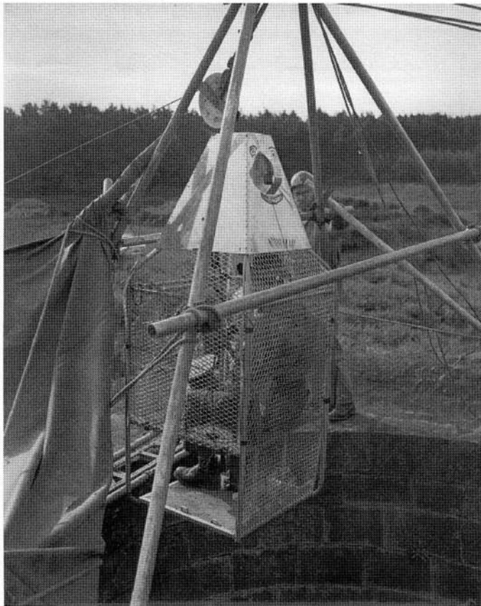
The cage mk.II on test over a 200ft. mine shaft in the Forest of Dean
